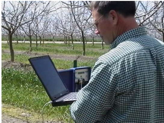
Data Logger Downloading to a Laptop
